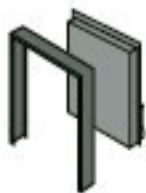
1: 1 spacer, freestanding or inset by 60mm.
