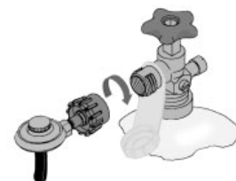
For Quick Connect cylinders, tighten clockwise
