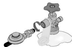
For POL cylinders, tighten counter-clockwise
