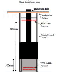
CLEARANCES BASED ON INSTALLATION HAWKWIND 200MM TRIPLE SKIN FLUE KIT.
