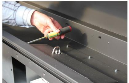
Remove the 'engine' by lifting up and to the left. This is still connected internally to the gas hose and power cables. Place engine just to the left within firebox as shown.
