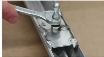
Step 3: Rivet the 4x spring clips onto the chassis of the appliance as shown
