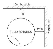
700mm minimum clearance is required if the rotation of the ErgoFocus is locked at 120° or 90° away from the wall. Locking the ErgoFocus so that the opening is fixed is an option available on purchase.
