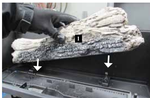
Logs 1 - fits over pins behind burner
