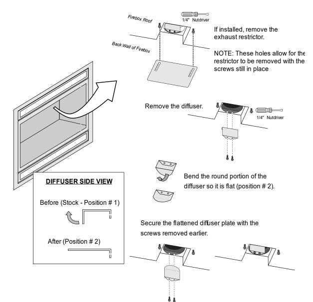
If needed, Replace the exhaust restrictor (see "Exhaust Restrictor Adjustment" for details).
