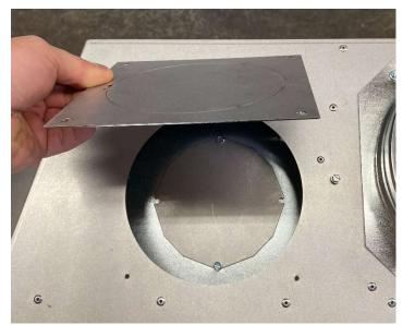
a) Remove the inner heat duct plate (2 screws - see picture below).
