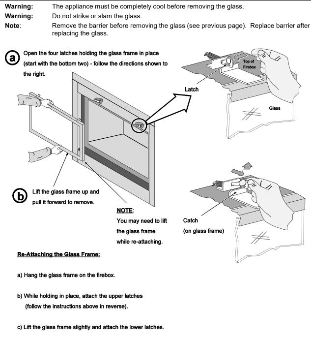
NOTE: Make ours the class frame is all the way in place – it should be fluch with
