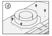
e) Line up the holes on the pipe shield flanges with the holes from the screws you just removed. Use the screws to attach the pipe shield to the top of the fireplace.
