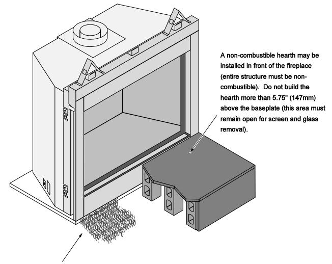
If installed near carpet or other combustible flooring, the fireplace must be raised so the base of the unit is above the carpet surface or flooring material.
