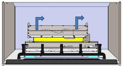
Lift the front burner, slide it to the right, and lift it from the firebox. When replacing the burner make sure it is properly located.
