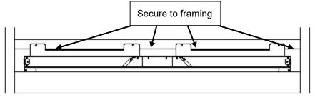
6 Re-attach the two rear mounting brackets (removed in step 6) to the bottom of the convection manifold. Leave the screws loose so the brackets can be positioned to the back of the chase. Secure the brackets to the chase using screws (not included). Tighten the screws securing the brackets to the manifold.
