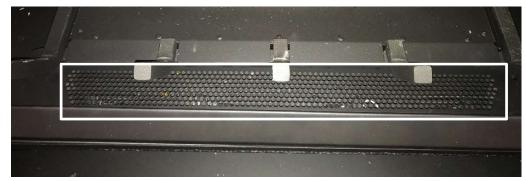
• Place a thick layer of the ember glass over the perforations making sure to cover all of the holes completely.
