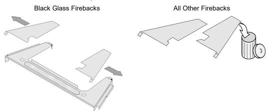
Rear Air Deflector (behind the rear log) Must be Removed (replace after firebacks in place)
