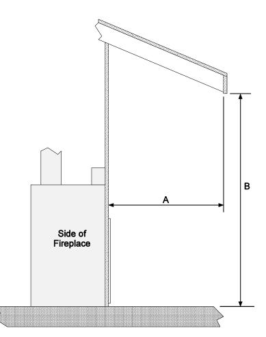
The overhang (A) must extend at least 1/2 the roofline height (B). Height is measured from the base of the fireplace.
