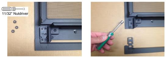
3. Remove and discard the lower trim (see photo above to the right). Replace the (3) nuts (both sides) to secure the hinge. Replace the screen assembly on the fireplace.
