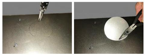
2 Grab on to the knockout with pliers and bend it back and forth until the remaining tabs break free. Discard the knock out plate.
