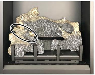
Log #7 Place log #7 as shown below. The charred end of log #7 rests on the burner. The right branch has a notch that aligns the log with the finger of the log grate. The upper end of log #7 rests on a groove in log #3.
