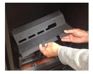
3. Remove the manifold covers. **NOTE:** Reinstall the manifold cover after changing the orifices
