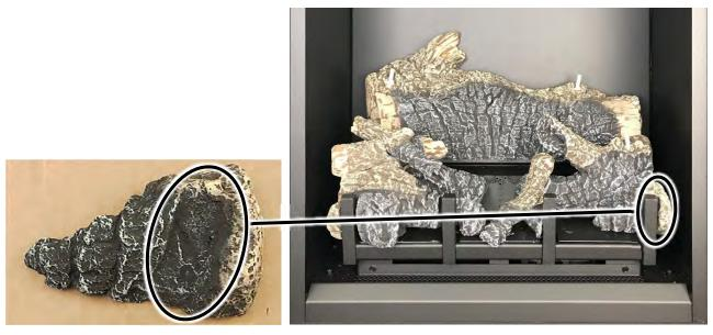
Log #9 Place log #9 as shown below. The hole on the bottom of log #9 fits over the pin on the left end of Log #1. The right end of log #9 rests on Log #7. There is a notch in the end of the log that rests on the finger of the log grate (see below).
