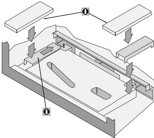
9 Place the two rivets into the burner holes shown below.
