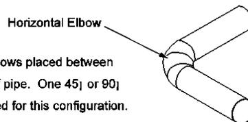
Horizontal elbows are elbows placed between two horizontal sections of pipe. One 45° or 90° horizontal elbow is allowed for this configuration.
