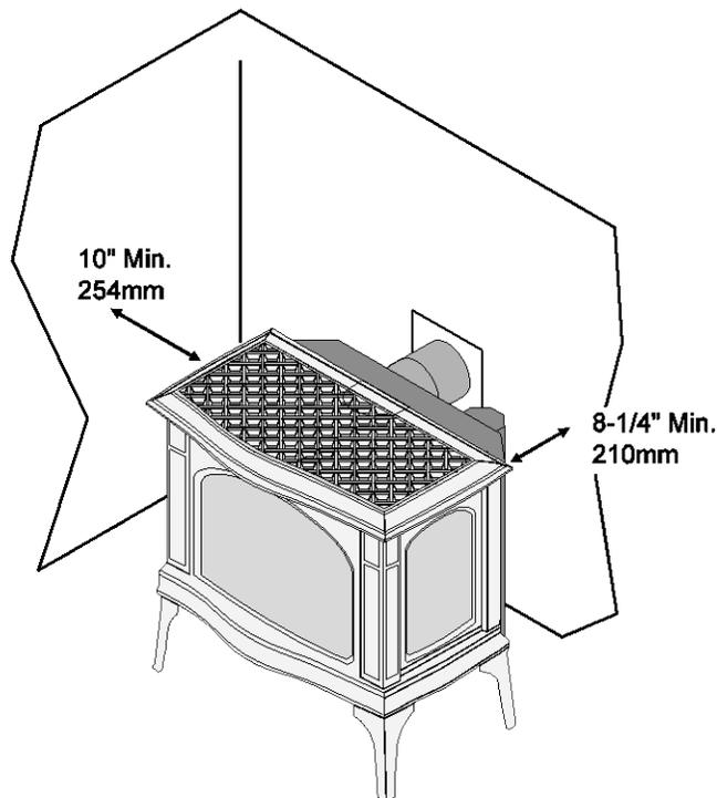
**i** Rear vent installations may not use an elbow with a horizontal termination. We recommend using a top vent configuration if placed in a corner
