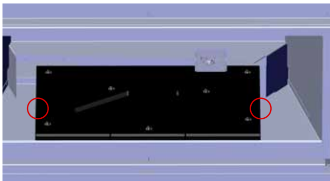
Diagram 2 - Burner Screw Locations
