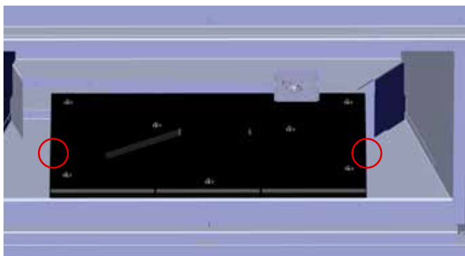
Diagram 2 - Burner Screw Locations
