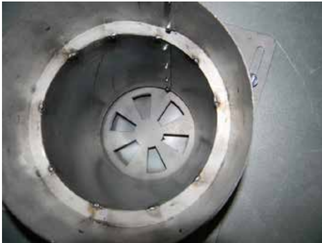
View with Cover Plate removed and unit adapter installed - primary air control now visible.
