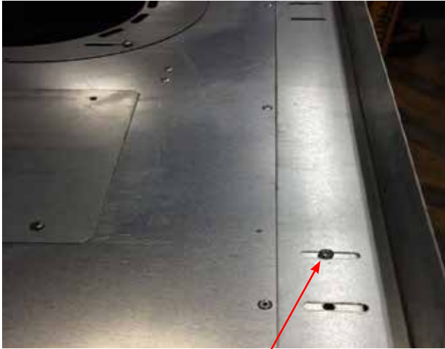
Nailing strip installed with slotted side on unit. The slot allows the movement of the nailing strip to be adjusted depending upon thickness of finish material.
