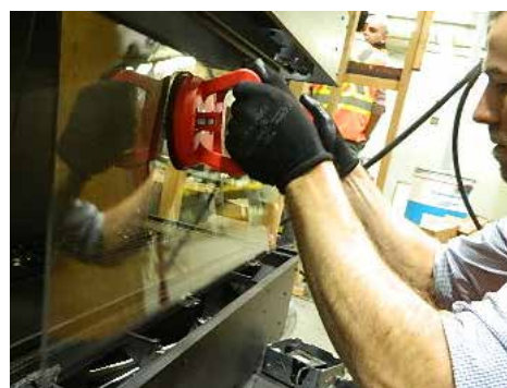
Handle front panel with supplied vacuum clamps
