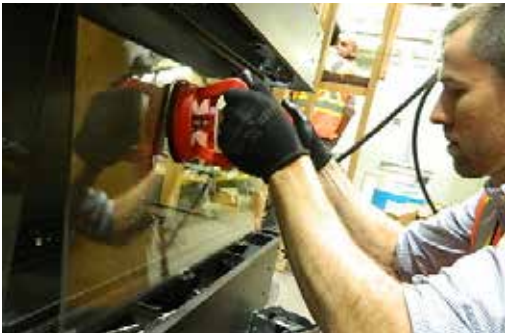
Handle front panel with supplied vacuum clamps
