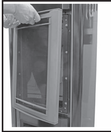
Figure 48: Removing mesh screen cover.
