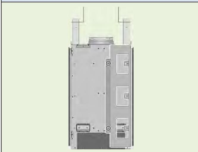
4. When the bracket is in the desired position, install the bolts that were removed in steps 1 & 2 and tighten the (3) bolts that the keyhole slots engaged.
