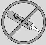
**WARNING:** Do not use adhesive to secure the facing. The high temperatures of the fireplace may cause adhesives to emit odors. Use mastic or thin-set (or other non-combustible, non-odorous adherent) to attach the facing.
