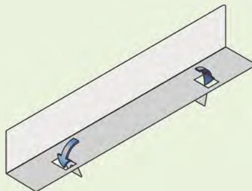
3. Set the header shield onto the standoffs with the 90° bend facing the middle of the fireplace. The tips of the standoffs will protrude through the heat shield.
