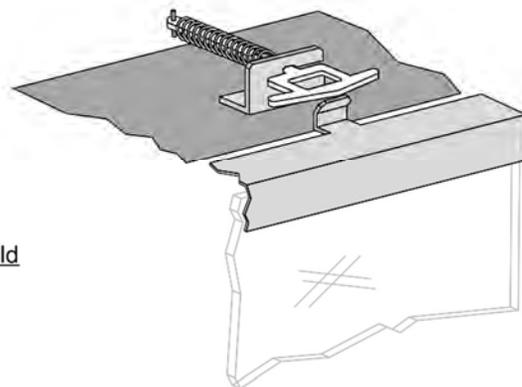
**NOTE:** Make sure the glass frame is all the way in place - it should be parallel with the front of the fireplace when installed.
