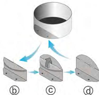
Remove the diffuser from the flue.
