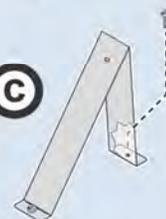
2. On the header shield, bend the two tabs downward.
