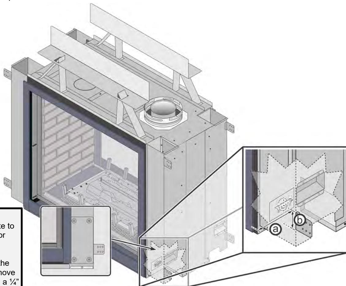
**NOTE:** There is a removable plate to allow access for making the electrical connection to the fireplace. Remove the plate using a 1/4" nut driver.
