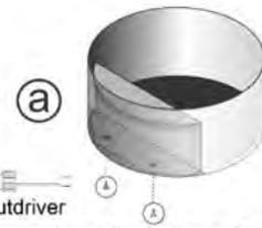
Reach up inside of the firebox and remove the (2) screws that secure the diffuser to the inside of the flue. Set the screws aside for reinstallation.
