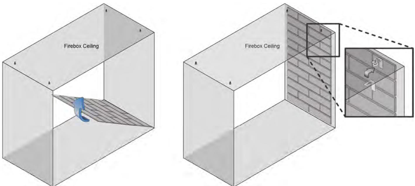
5. Restore the fireplace to the correct configuration (make sure to reinstall the baffles)
