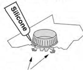
Bend the tabs on the bottom of the starter collar up to lock it in place.
