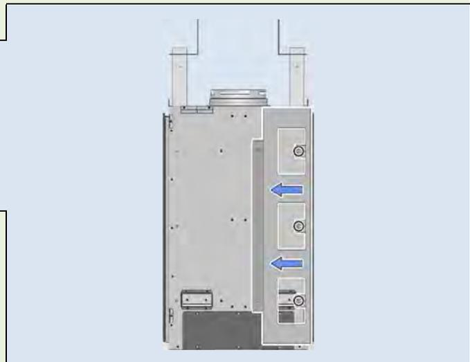
3. Place the keyhole slots on the centering bracket over the three bolts along one of the edges of the fireplace. With the keyholes over the loosened bolts, slide the bracket toward the center. The position of the standoff is dictated by the desired way to apply the finish material (see "Standard vs Extended Position" on page 33).
