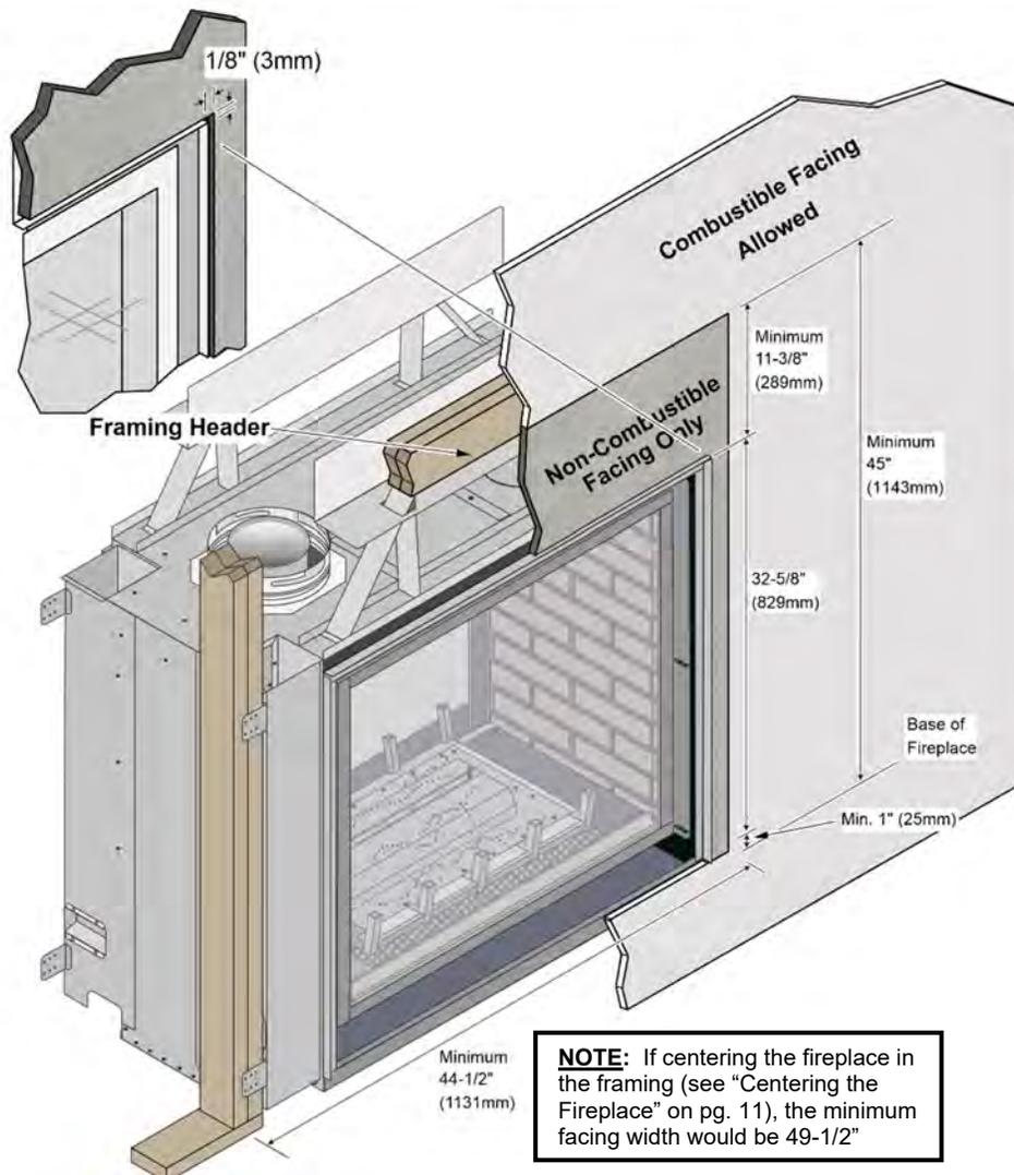
**NOTE:** If centering the fireplace in the framing (see "Centering the Fireplace" on pg. 11), the minimum facing width would be 49-1/2"
