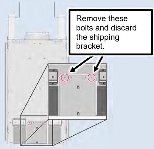
2. Loosen (but do not remove) the (6) bolts along the outer edge of the end of the fireplace marked with black circles. Remove the (2) bolts marked with red circles to the right. Set the bolts aside for reinstallation.
