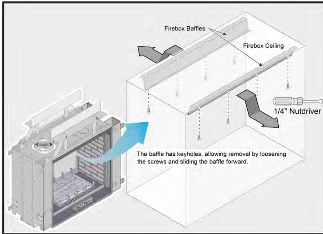
3. Remove the (4) fireback clips (2 on each side) from the ceiling of the fireplace (see illustration below).
