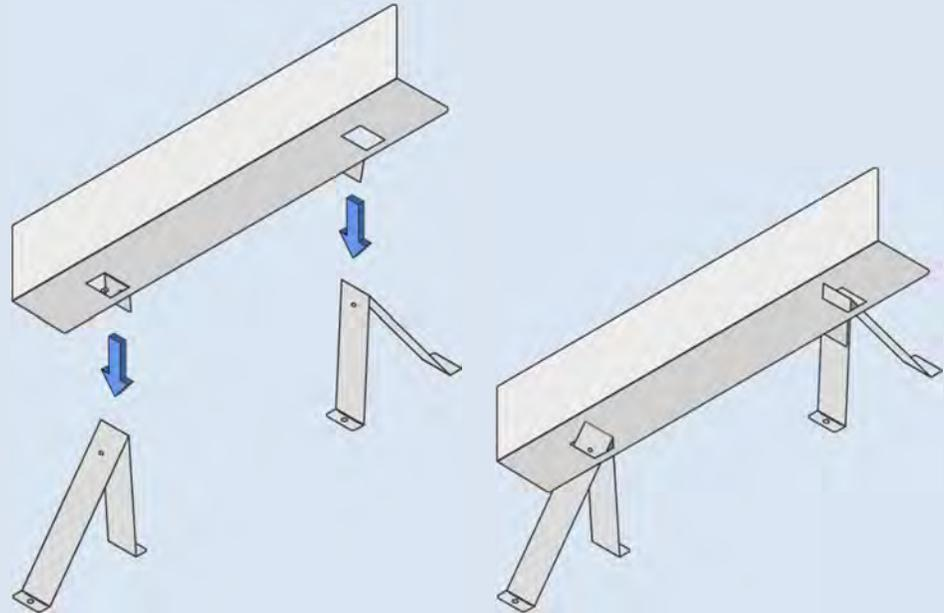
4. Attach the heat shield to the standoffs by aligning the holes on the heat shield tabs with the holes in the header standoffs and secure using the included screws.
