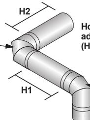
Horizontal length is calculated by adding both lengths of horizontal run (Horizontal Length = H1 + H2).
