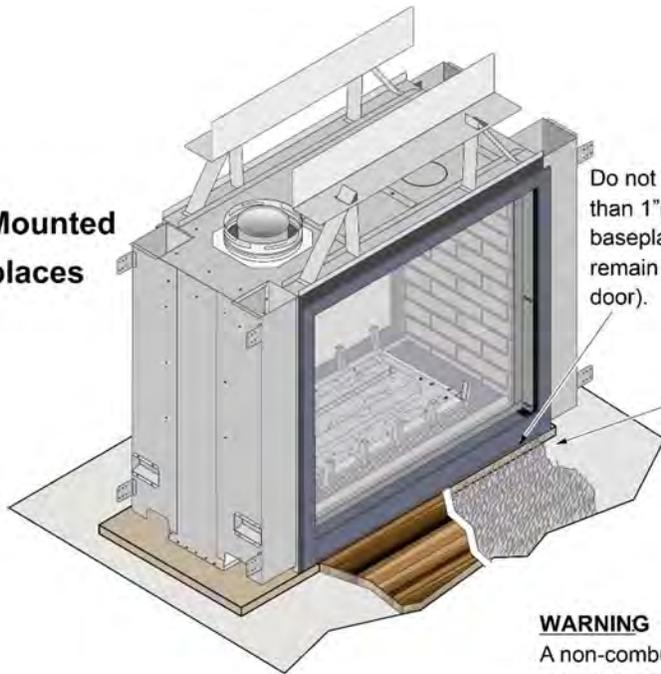
Do not build a hearth more than 1" (25mm) above the baseplate (this area must remain clear for the access door).
