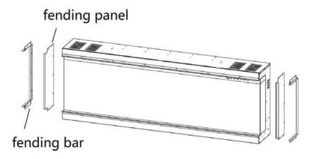
**3.** Fix back the fending bars after the panels are removed.
