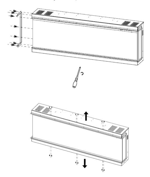
**5.** Fix the brackets with the screws in the previous step.
