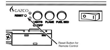
Resetting of the remote control is necessary if the appliance operates wrongly due to external interference signal and the remote control is not in use.
