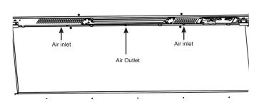
Dust build-up can inhibit efficient performance of the fan and lead to the safety cut-out operating.
