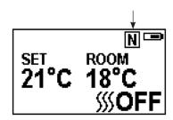
Press the '+' or '-' button to adjust the setting temperature from 17 °C to 25°C.
