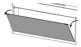
Remove and wash the fuel effect to remove any dust particles. Alternatively clean with a lint free duster.
