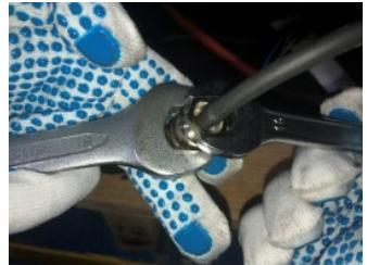
6. Then feed the power cable through the exit hole and the secondary locking nut is tightened on the outside, securing the power cable to the appliance, as seen bellow.
