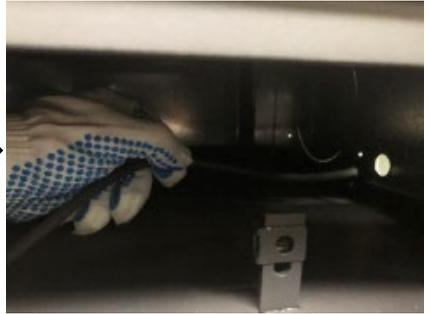
4. Feed the cable until the cable keeper reaches the exit hole. Holding the cable keeper in place, adjust the power cable length such that there is sufficient slack between the exit hole and the ventilation kit, as shown bellow.
