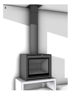
Fit the fascia components back to the console. Install the ceiling plate to cover the hole for the flue pipes. Complete the project with any remaining fixtures and finishes.
