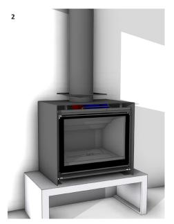
Secure the freestanding console to the floor, base or plinth. Install the DF700 fireplace into the freestanding console connecting the flue spigot plate to the fireplace. Connect gas supply and powerflue electrical cable. Connect power supply to wall outlet. Complete commissioning of the fireplace and flue.
