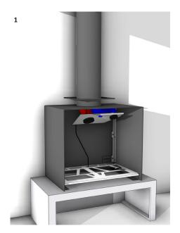
Locate the freestanding console in the desired location, complying with all clearances. Allow for an electrical outlet within 1m. Remove the console fascia and set aside. Install the black rigid liners to the console, run the twin flexible flue pipes and connect to the removable flue spigot plate. Conenct the powerflue electrical cable at both ends.
